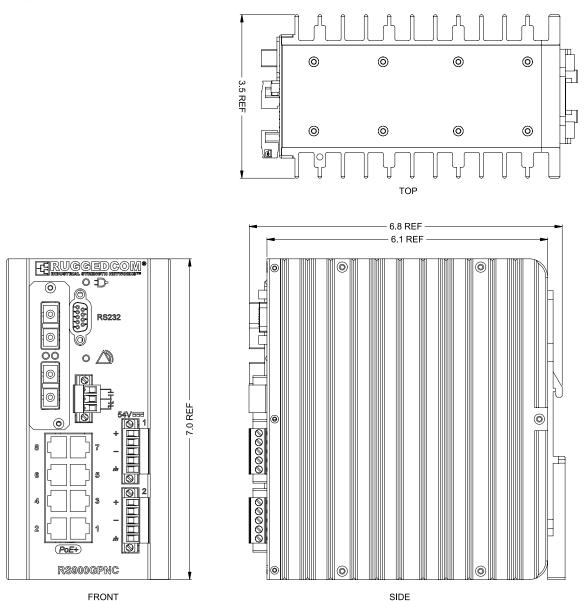
Figure 3.1. RS900GP Physical Dimensions
